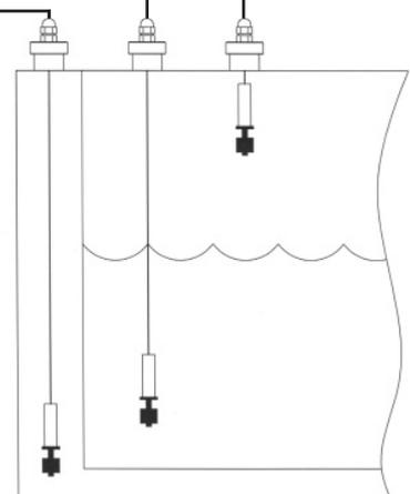
Due to the reclassification of diesel which is now classed as a flammable liquid under the CLP Regulations, the Hytek tank alarms have been ATEX certified for use with diesel.
