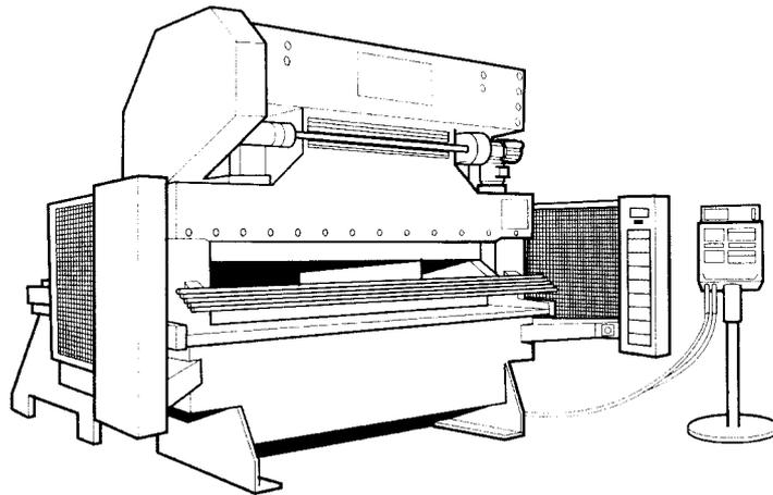
**Figure 3** Photoelectric device fitted to a press brake
