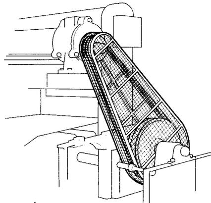
**Figure 1** Fixed enclosing guard
